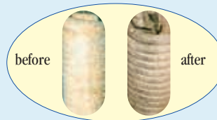
Scale reduction in heat exchangers
